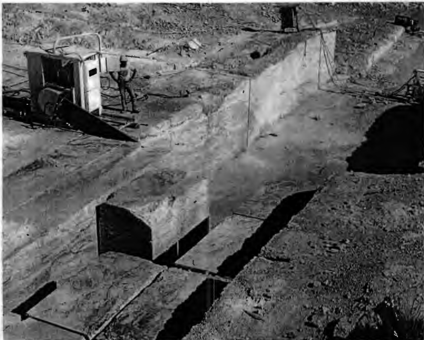
FIGURE 1—Scheherazade quarry at New Mexico Travertine quarries west of Belen, New Mexico. Diamond-impregnated belt saw in operation cutting 1 1/2-inch channel as deep as 10 ft. Wire saw at upper right is "pulling the floor" on block previously cut by belt saw. Photograph courtesy of Rocky Mountain Stone. (Contents on page 50)
